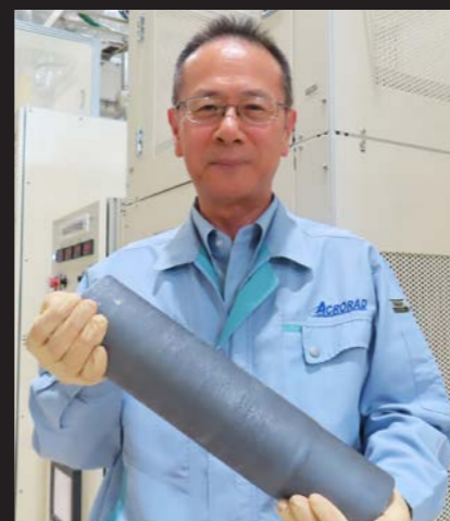
▲ A photon-counting CT system (left) uses a new type of detector containing cadmium telluride. This was only possible because of advances in producing high-quality cadmium telluride, pictured here being held by the detector material's developer Ryoichi Ohno (right).
