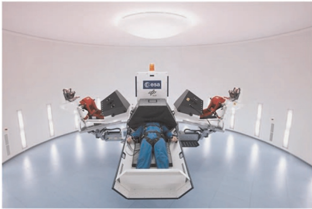
Figure 4. European Space Agency short-arm human centrifuge at DLR (Cologne). Maximum radius at outer perimeter: 2.8 m; maximum centrifugal acceleration: 4.5 g (floor level, test subject height: 1.85 m); number and type of nacelles: two beds, two seats; maximum overall payload: 550 kg (Credit ESA and DLR).
