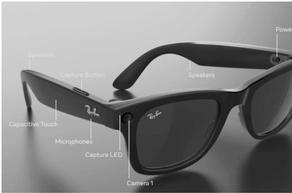
Fig. 1 Technology components of Ray-Ban Meta smart glasses. Reprinted without changes from Laurent C, Iqbal, M.Z., Campbell, A.G. Adopting smart glasses responsibly: potential benefits, ethical, and privacy concerns with Ray-Ban stories. AI Ethics. under Creative Commons Attribution 4.0 International License http://creativecommons.org/licenses/by/4.0/ .
