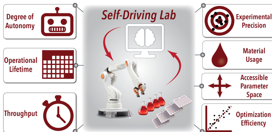
Fig. 1 | Key metrics for quantifying performance in SDLs. The metrics illustrated include degree of autonomy, operational lifetime, throughput, experimental precision, material usage, accessible parameter space, and optimization efficiency.
