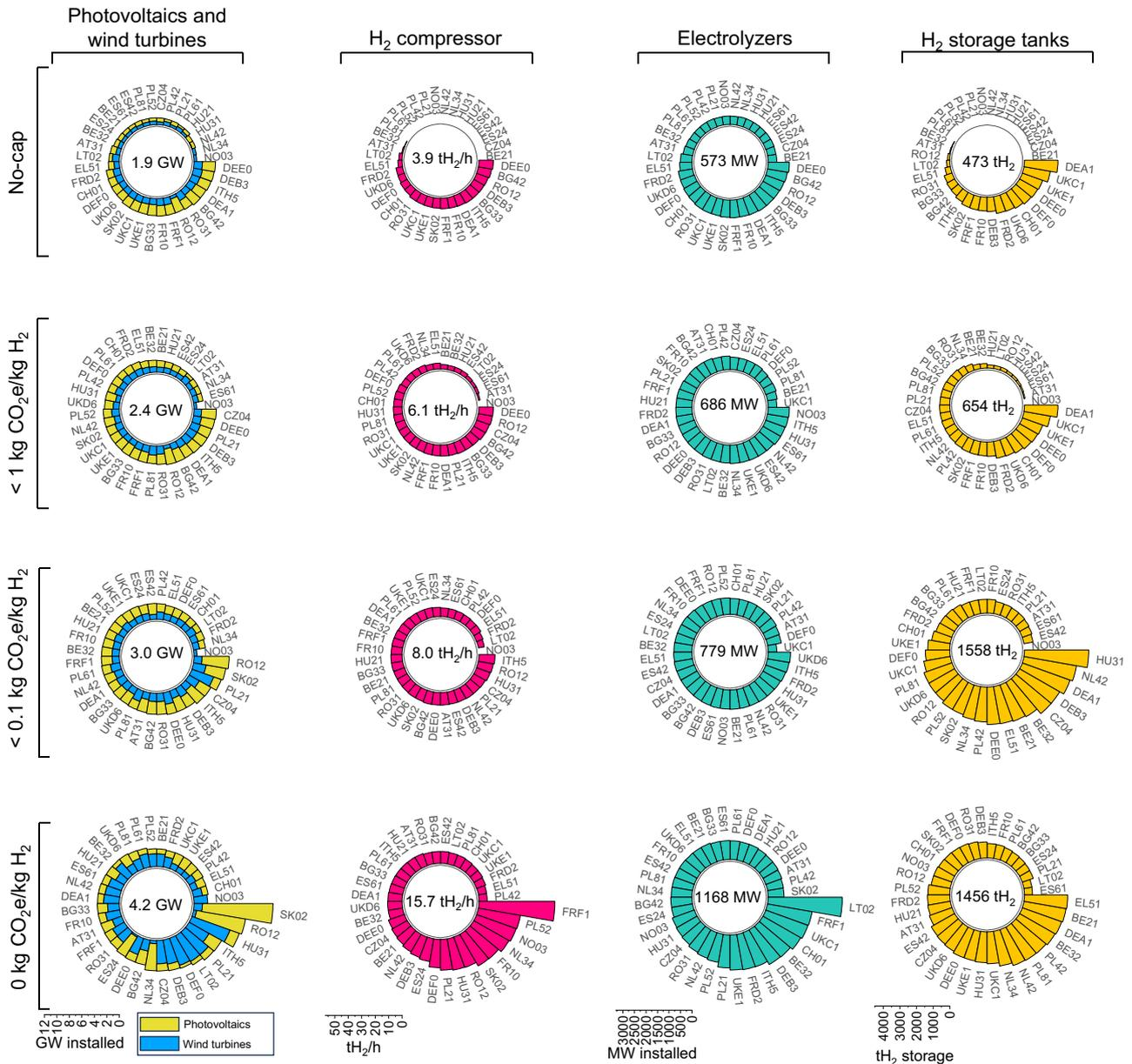
**Fig. 3 | Optimal electrolytic hydrogen production system (EHPS) design across Europe.** Regions coded according to the NUTS-2 level of the Nomenclature of Territorial Units for Statistics (NUTS) system (Supplementary Table 1) and ordered by installed capacity. Values inside the spirals refer to the mean installed capacity of the respective component in European plants given emission constraints (caps) on the lifespan well-to-gate carbon dioxide equivalent (CO<sub>2</sub>e) content of
