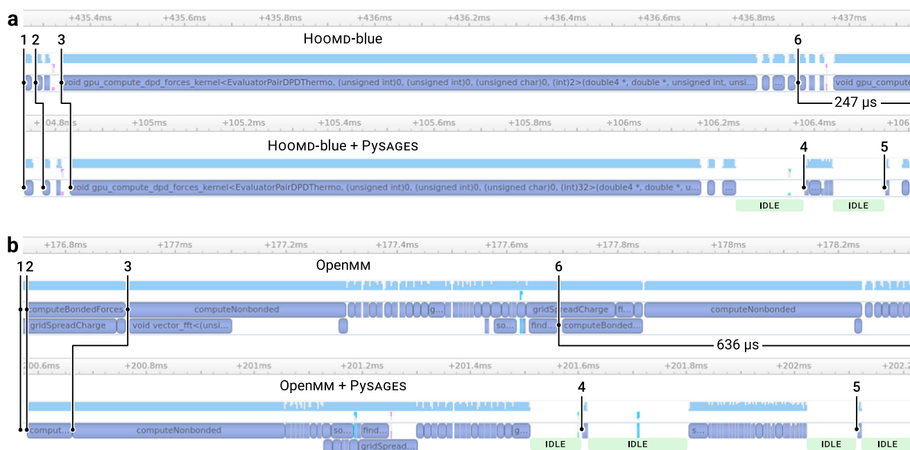
Fig. 9 Profiled timelines for a single-time step of unbiased and biased execution with HOOMD-blue and OpenMM. The profiles were recorded with Nvidia Nsight systems on an Nvidia V100 GPU. Light-blue represents the GPU activity while dark-blue represents individual CUDA compute kernels. The numbered lines indicate the same compute steps in all simulations: (1) start of integration step, (2) compute of bond forces, (3) pair-wise forces, (4) calculation of the CV, (5) addition of the harmonic biasing force to the backend, and (6) end of the integration step. (4) and (5) are PysAGES only and are executed on the GPU. We observe GPU idle time during the PysAGES Python coordination with GPU-JAX/CuPy (green bar), but note that there is no memory copies even within the GPU memory. a 1.8 ms of recorded HOOMD-blue execution. The top row shows a vanilla HOOMD-blue simulation step, while the bottom row shows a PysAGES/HOOMD-blue simulation with harmonic biasing of a center of mass CV. The additional time for CV biasing per time step is 247 \mu\text{s} . b 1.6 ms recorded execution time line of an OpenMM OPLS simulation of 40,981 particles as polymers with PME summation for long-range Coulomb forces. OpenMM works with asynchronous GPU kernel execution, which leads to less linearly-sorted timelines. Overall, the performance degradation is more pronounced with OpenMM compared to HOOMD-blue.
