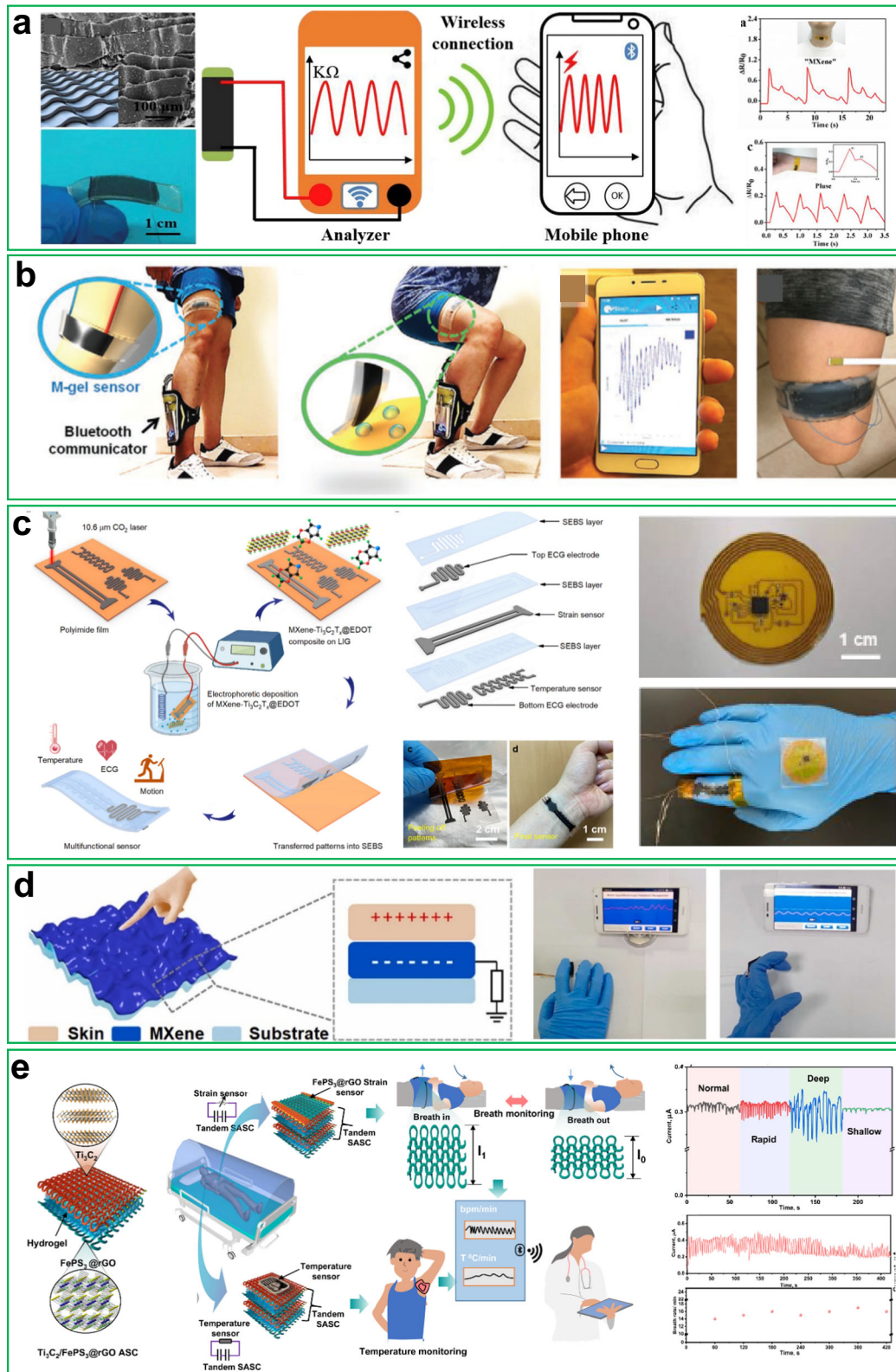
Fig. 4 Wearable strain sensor. a Polyaniline@ Ti_3C_2 -based flexible strain sensor with a tile-like stacked structure for wireless detection of artery pulse and phonation. Reprinted with permission 51 . Copyright 2020, Elsevier. b Wearable wristband based on a Ti_3C_2 hydrogel strain sensor and Bluetooth module wrapped around a human thigh during a workout to measure the degree of muscle tiredness. Reprinted with permission 18 . Copyright 2021, Wiley. c Ti_3C_2 @3,4-ethylenedioxythiophene/graphene composite-based wireless multifunctional sensors for strain, temperature, and heartbeat monitoring. Digital images represent the wearability and skin comfort of sensing system. Reprinted with permission 52 . Copyright 2022, Springer Nature. d Schematic illustration of the crumpled Ti_3C_2 film and the self-powered real-time monitoring system that wirelessly transmits varied degrees of finger bending and pressing signals to the smartphone. Reprinted with permission 55 . Copyright 2022, Elsevier. e Remote health monitoring system based on an integrated FePS_3/rGO strain sensor and a flexible supercapacitor for real-time breathing rate and body temperature monitoring. Reprinted with permission 14 . Copyright 2022, Springer Nature.
