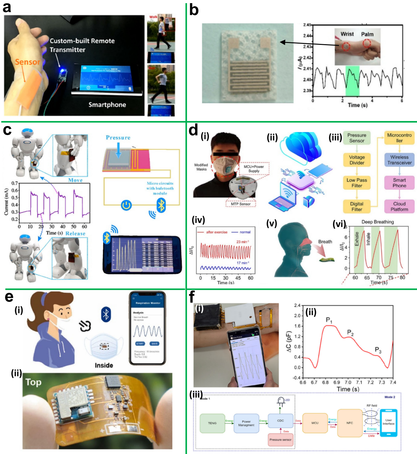
Fig. 3 Wearable pressure sensors. a Image of graphene-based pressure sensor assembled on the wrist to remotely monitor pulse rate during walking and jogging. Reprinted with permission 40 . Copyright 2019, Elsevier. b \text{Ti}_3\text{C}_2 -based pressure sensor for wireless wrist pulse monitoring. Reprinted with permission 41 . Copyright 2019, American Chemical Society. c \text{Ti}_3\text{C}_2 -based pressure sensor to monitor movements of the robot and detected current signals transfer to the mobile device via Bluetooth communicator (Reprinted with permission 16 . Copyright 2020, American Chemical Society. d Smart face mask for wireless detecting opiate overdoses and monitoring respiration; (i) image of a smart mask with integrated \text{Ti}_3\text{C}_2 pressure sensor unit, power supply unit, and wireless data transmission unit, (ii, iii) a schematic and block diagram of wireless respiration monitoring system, (iv) respiration cycle monitoring before and after activity, (v) diagrammatic representation of human exhaled air detection, (vi) monitoring deep breathing cycle. Reprinted with permission 42 . Copyright 2021, American Chemical Society. e MWCNT@ \text{Ti}_3\text{C}_2 fabric-based smart mask for respiration monitoring; (i) schematic view of an integrated mask with detection tag and wireless data transmission and (ii) front and back side images of respiratory detection tag. Reprinted with permission 43 . Copyright 2022, Elsevier. f Wearable \text{Ti}_3\text{C}_2 -based remote health monitoring system; (i) photograph of wearable health monitoring system assembled on the wrist and recorded pulse transferred to a smartphone, (ii) zoom view for single wrist pulse, and (iii) system block diagram for remote health monitoring. Reprinted with permission 47 . Copyright 2022, Elsevier.
