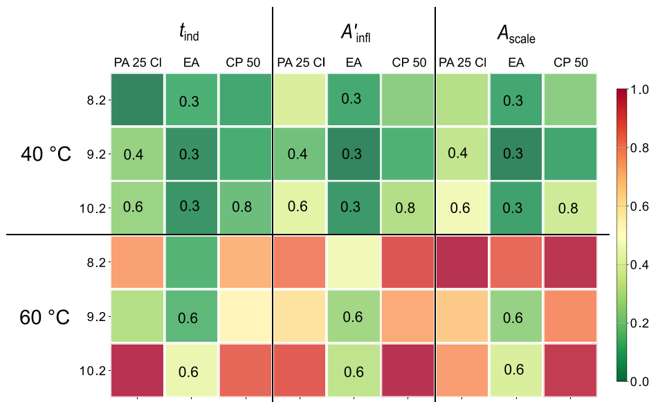
Fig. 6 | Performance heat map calculated for different additives. The heatmap includes data of three different additives (Sokalan® PA 25 Cl, etidronic acid and Sokalan® CP 50) at a maximum concentration of 1 ppm. For conditions where precipitation was completely suppressed at 1 ppm, the highest possible concentration of the additive is given in the respective box.
