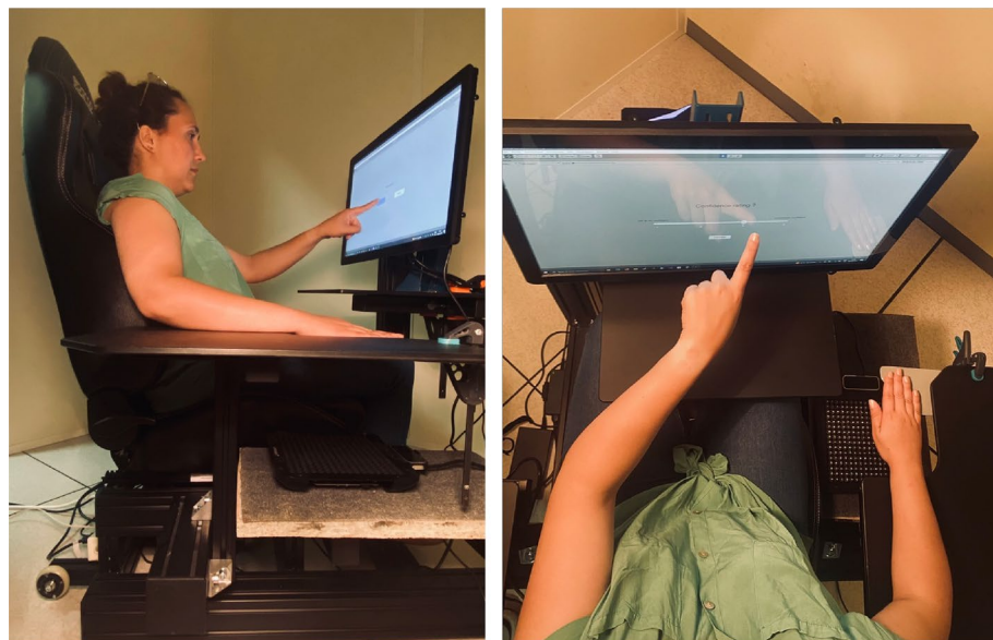
Figure 4. Overview of the experimental setup and participant positioning. Stimuli were delivered using an array of ultrasound actuators positioned 20 cm below the participant’s right hand.
