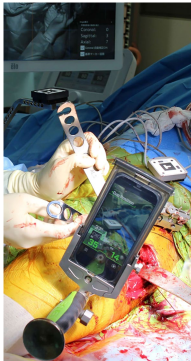
Figure 5. In the portable augmented reality (AR)-based navigation system, the smartphone is attached to the cup impactor. The smartphone recognizes the AR marker attached to the fixation pins at the pelvis. The display of the smartphone shows the radiographic inclination (RI) and radiographic anteversion (RA) of the cup.
