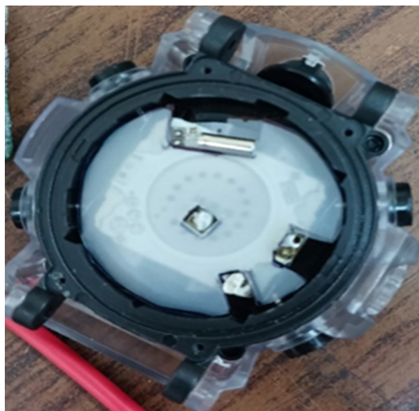
Figure 14. Terminals of the Watch Circuit.
