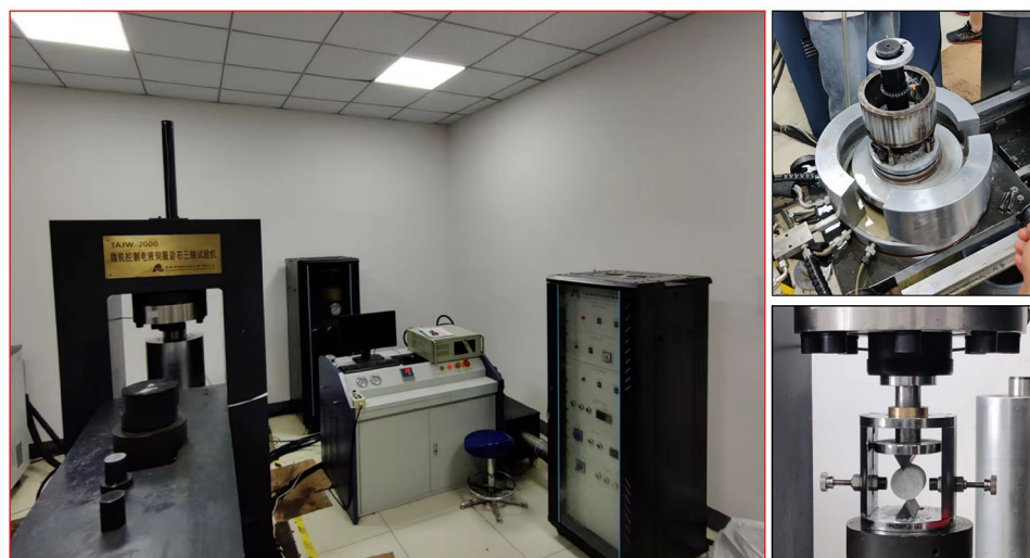
Figure 5. TAJW-2000 rock compression testing apparatus.
