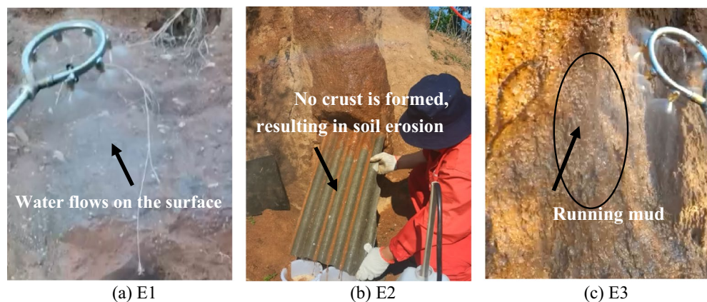
Figure 11. Field erosion resistance test.
