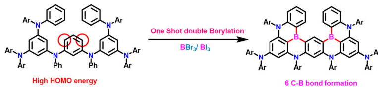
Fig. 6 Possible synthetic routes of double borylations. The synthetic pathways utilized for most of the DB-MR-TADF emitters.
