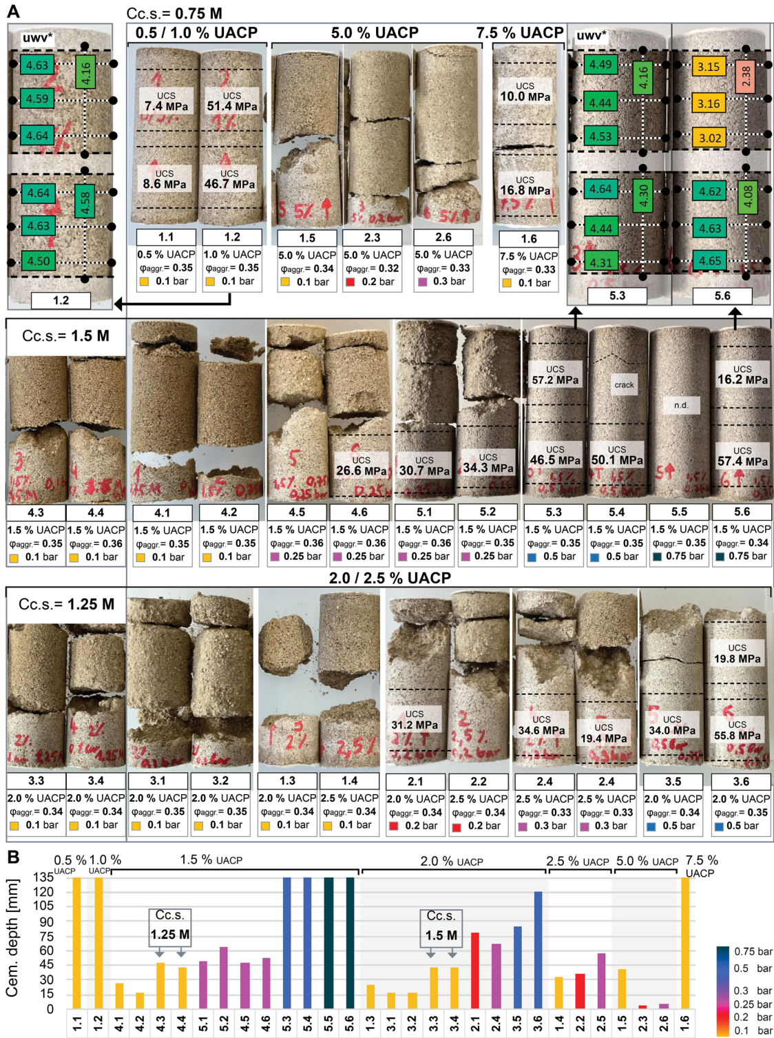
Fig. 4 Biomineralized specimens produced in test series 1–5. A The UCS-measurements of the cut samples and the positions of the cuts are marked in the images of the specimens. The ultrasonic wave velocity measurements (*uwv, [km/s]) at the marked points are shown in the enlarged images of the specimens 1.2, 5.3 and 5.6. B The cementation depth diagram of all produced specimens sorted according to the amounts of UACP and applied pressures.
